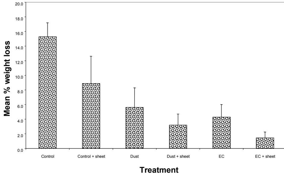
**Figure 7: Mean weight losses ( $\pm$ sem) from maize cobs stored in maize cob barns for six months and given various protective treatments which included dilute dust (dust) or emulsifiable concentrate (EC) formulations of Actellic Super with or without a plastic sheet (sheet) over the barns (n = 3).**
