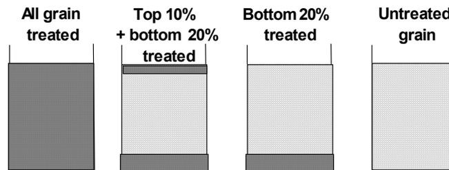
**Figure 8 - Treatments tested in farm stores using Zimbabwe maize grain**
